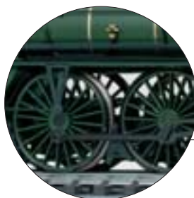
Immense driving wheels - diameter in real life: 2.20 meters / 86-5/8 inches
