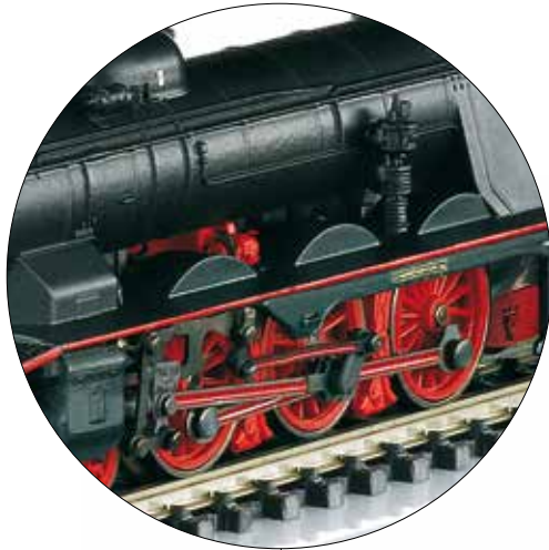
Finely executed and detailed valve gear and side rods
