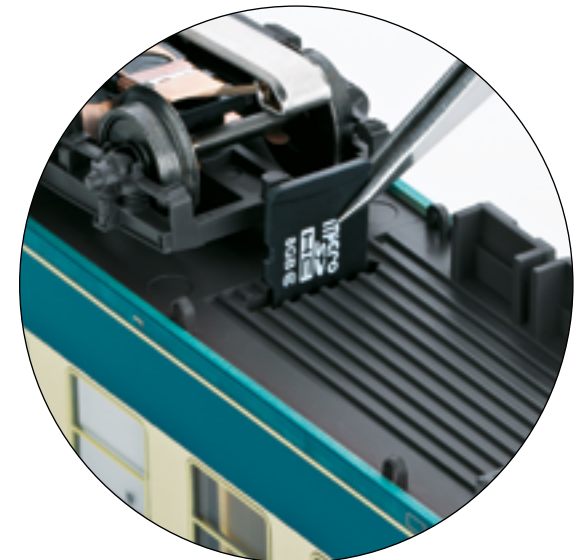
Cleverly hidden! The plug-in for the microSD card
