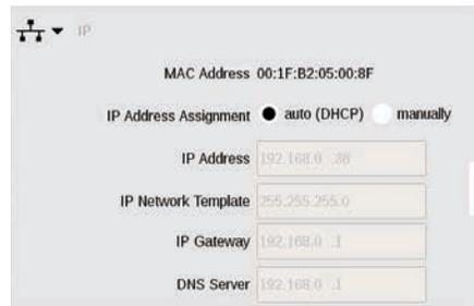
This option is available when you connect your Central Station 3 to your router with an LAN cable. Here you have the choice whether the CS3 is to obtain the necessary network addresses from the router or whether you are to enter the data manually.
