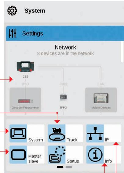
IP setting in case an LAN cable is connected.
