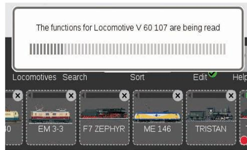
**Setup:** Place the mfx locomotive completely on the track. mfx locomotives can be done on both the main track and on the programming track.
