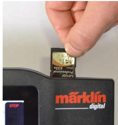
With an SD card (SDHC), you can expand the internal memory (4 GB) by up to 32 GB. All you have to do is plug the card into the card slot. You do not have to make any other settings.
