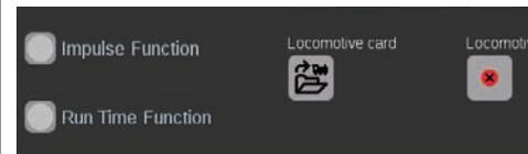
**Writing:** Insert the locomotive card into the card reader as shown. Tap on the symbol „Locomotive card“ in the tab „Set Up“ in the locomotive settings: The CS3 will write the locomotive data on the locomotive card.
