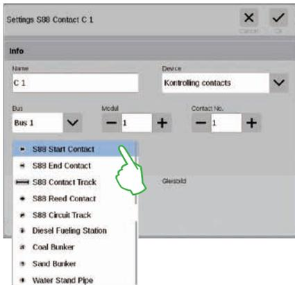
In the drop-down menu „Type“, select the type of feedback contact installed: contact track, reed contact, or circuit track.
