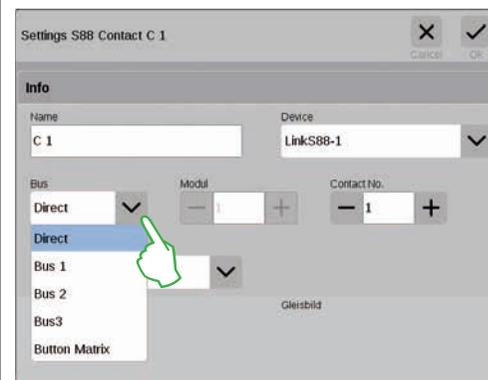
When you are using the Link S88, feedback contacts can be connected in the following ways:
