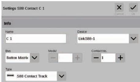
You can use the L88 for a button matrix, such as for a track diagram control screen. Up to 64 buttons (32 solenoid items or 64 routes) are supported. You enter the switching points belonging to them in the field „Contact No.“.
