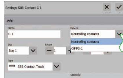
You set the device to which the feedback contact is connected in the drop-down menu „Device“. On the CS3 plus you will find here the option „GFP3-1“ that corresponds to the S88 connection on the underside of the device (left image). On the CS3 (60226) feedback modules are connected by means of the Link S88 (see below).
